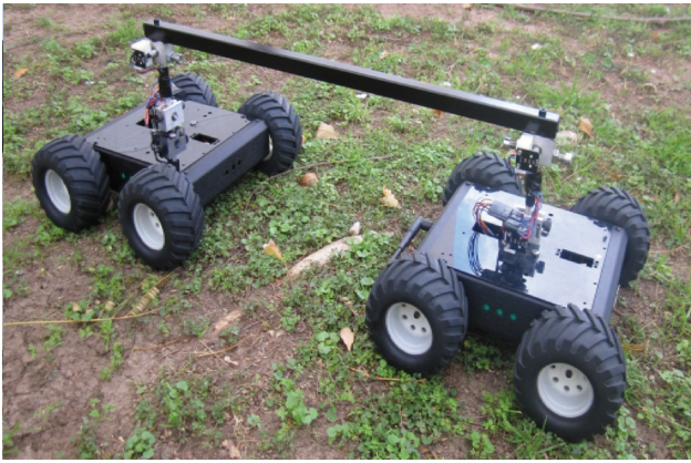
Fig. 1. The research prototype. Platform size is 34 \times 40 \times 25 cm with a 64 cm long connecting beam.
