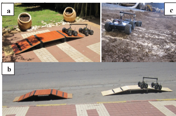
Fig. 10. Experiments setup. Single bump (a) flat wooden plate placed of a flat road. Multiple bumps (b) the first bump is lower and longer than the second bump. Rough terrain (c) the gravel ground is constantly changing making it difficult for mapping. The terrain includes three different bumps (height and width).
